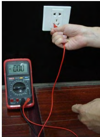
Appendix Figure 7-7 Check neutral cable connection
